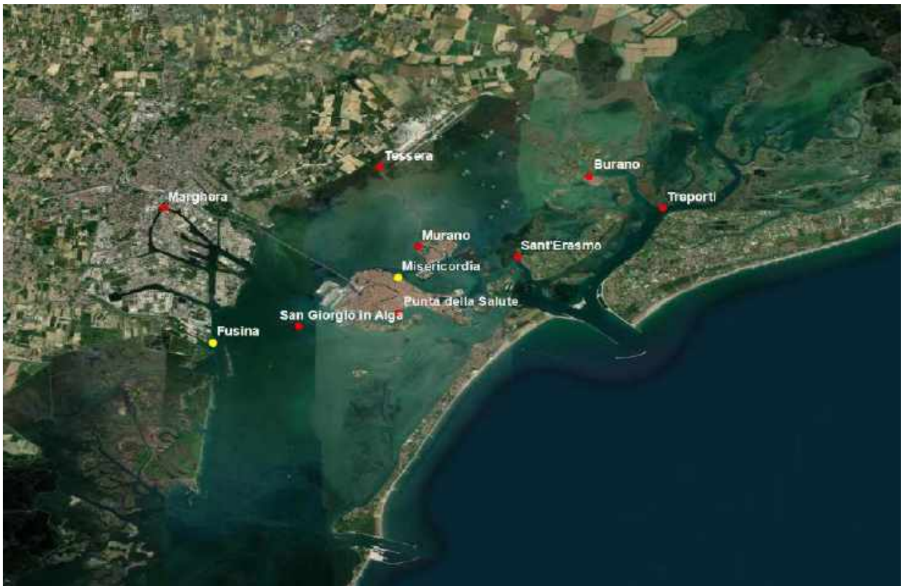
Figure 56. Tide gauges used for model calibration and validation. In red stations from “ISPRA-Venezia”, in yellow stations from “Città di Venezia”.
