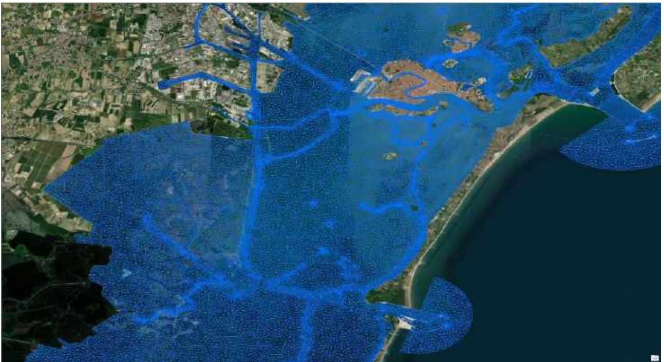
Figure 47. Mesh details: central lagoon area.
