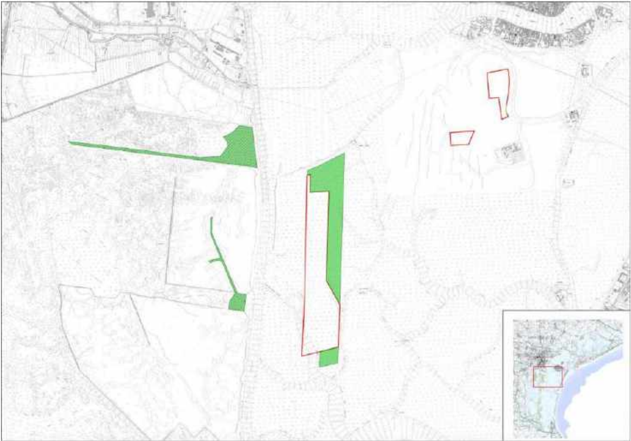
Figure 38. Central Lagoon: differences between the surfaces of the required concessions (April 2018) and those of May 2015 (red contour) are shown in the colors of the map. The areas to abandon are shaded in yellow, and the areas of new demand are shaded in green (after Piano d'Uso delle Aree in Concessione per la Venericoltura, [24]).
