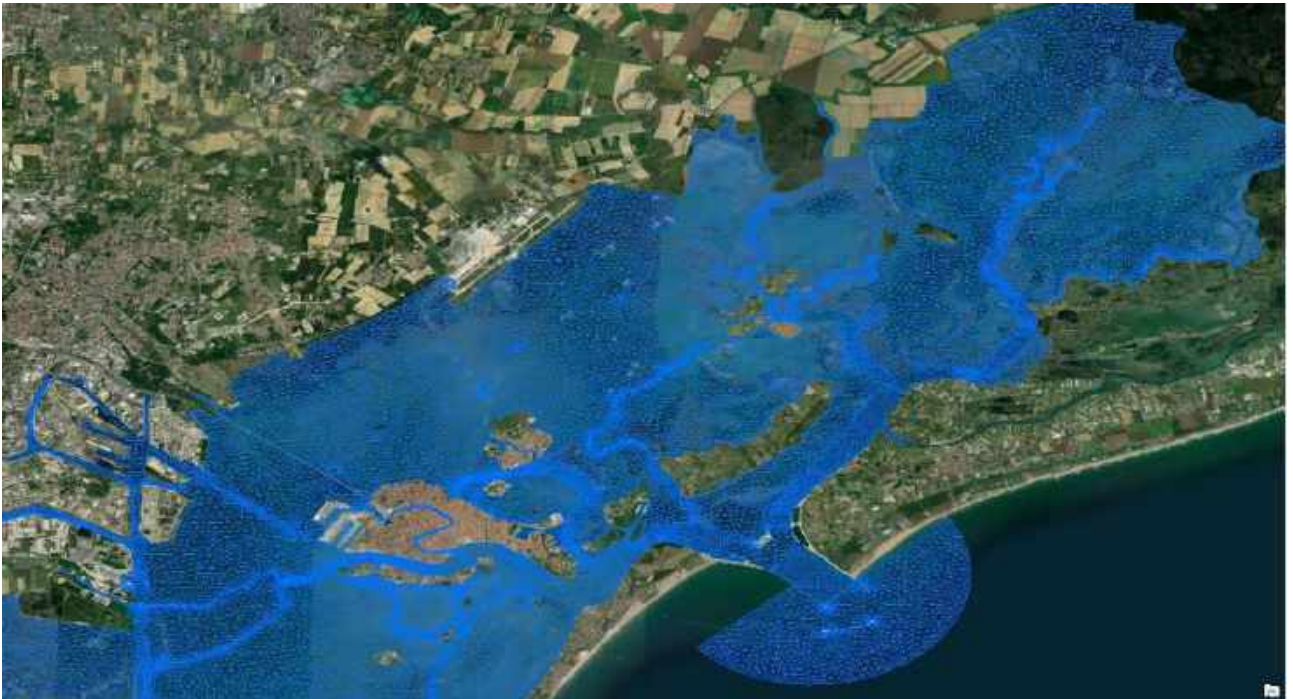
Figure 46. Mesh details: northern lagoon area.
