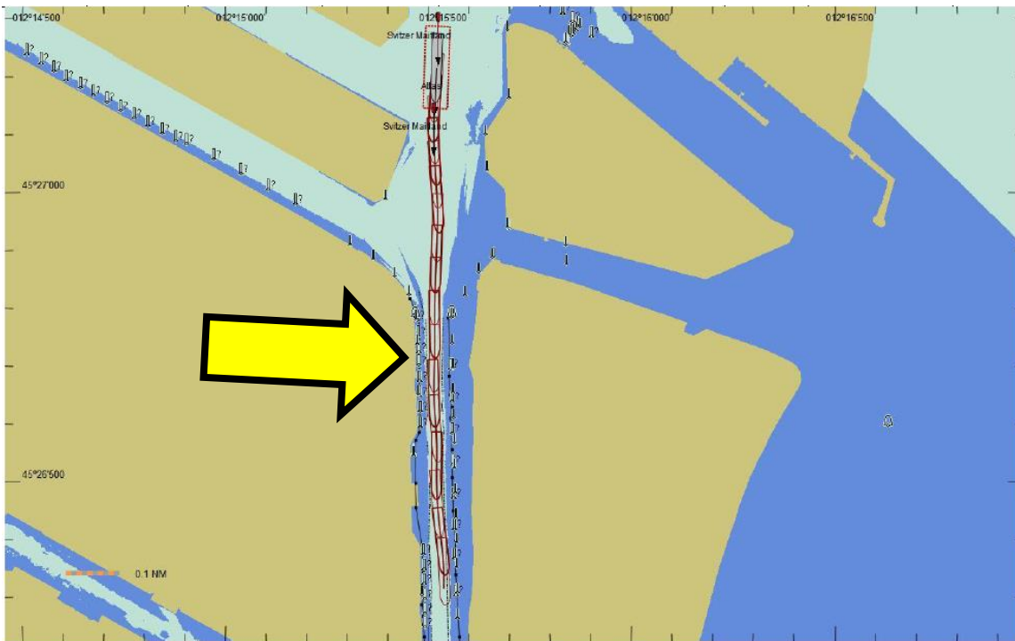
Figure 3.6. Grounding area south of turning basin #3 (run 502).
