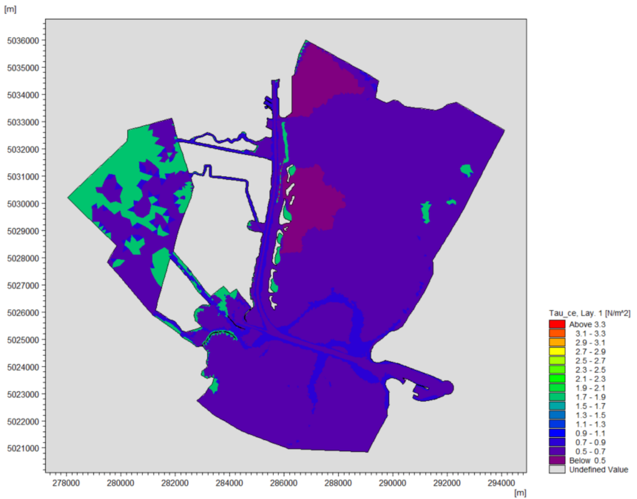
Figure 2.8 Updated map of critical bed shear stress for erosion of top sediment layer.
