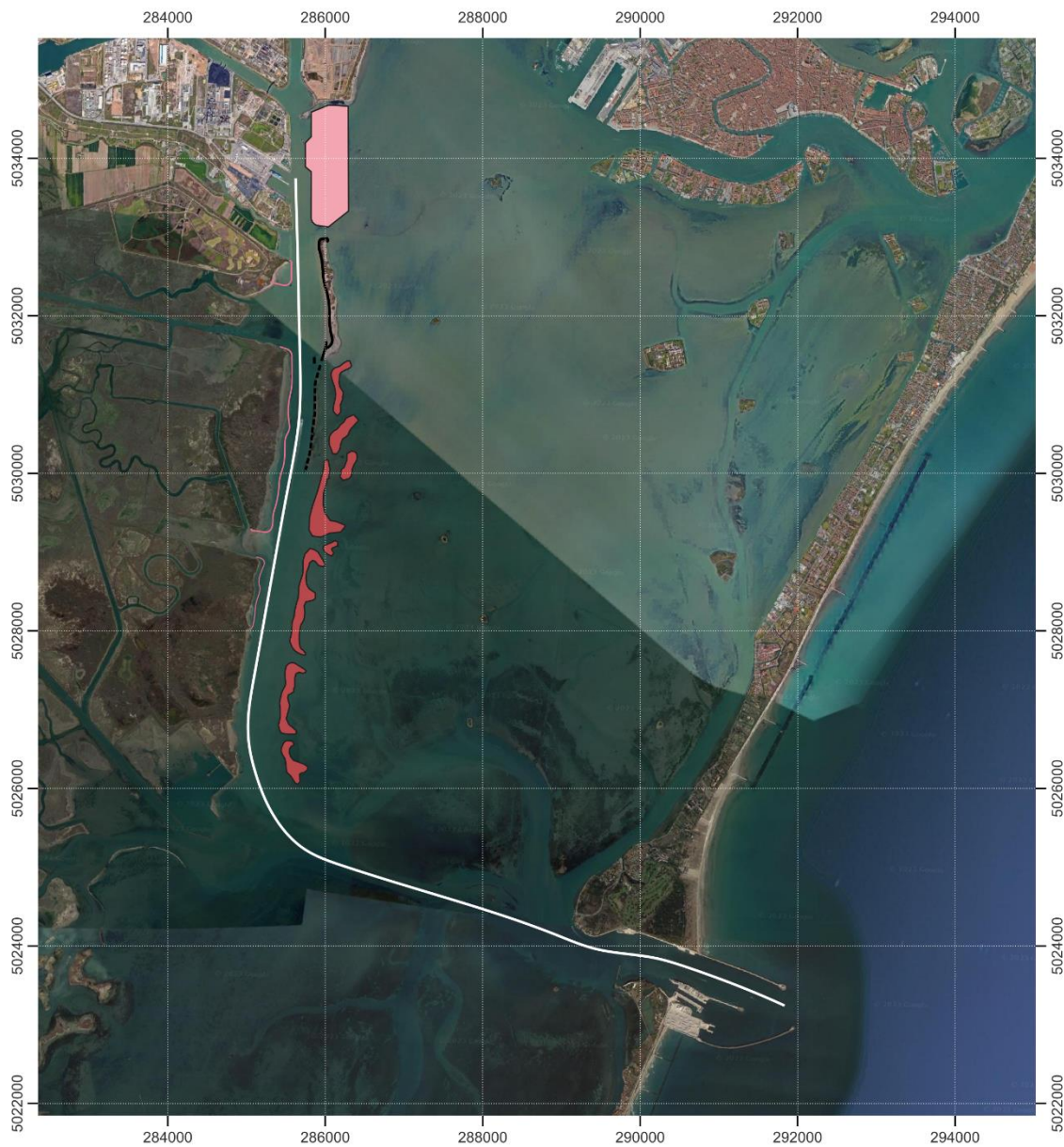
Figure 2.2 Overview of structural features in the new channel layout. Coloured polygons indicate the implemented structures. The white line indicates the vessel trajectory.
